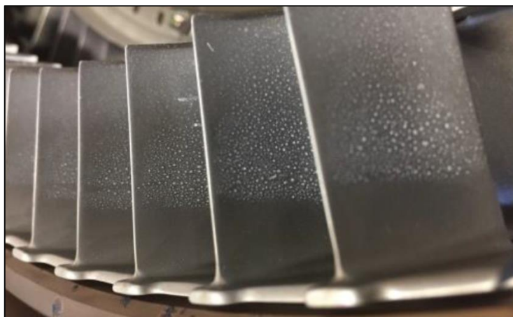
Photo No. 1: White Crystalline Deposits on Stage 4 Stator Vanes ( Engine Manufacturer )
